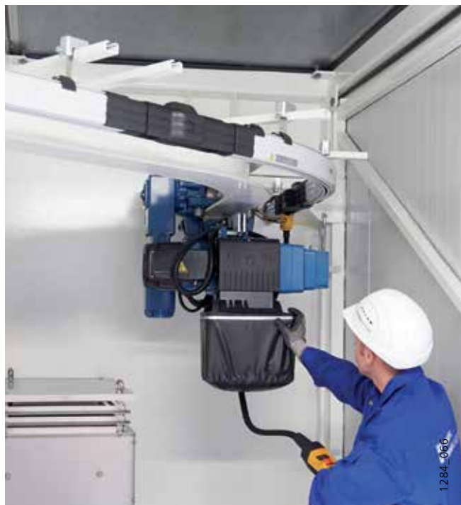
Articulated trolleys: low headroom dimension with infinitely variable speed
