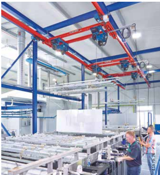
Double chain hoists operating in tandem with four chain lead-offs
